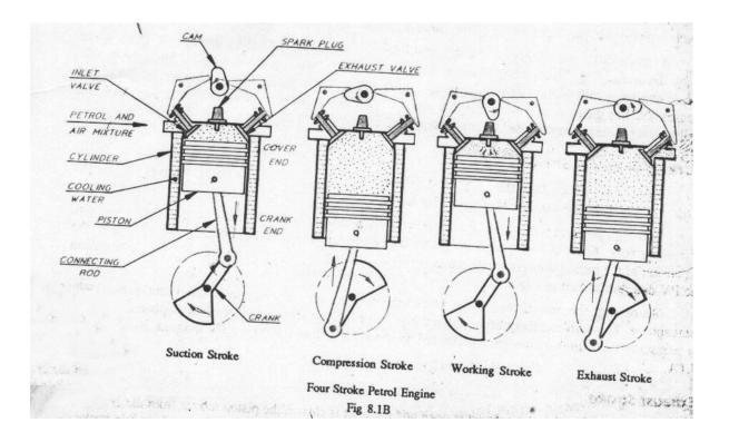
It operates on theoretical Otto cycle. Here cycle is complete is completed in two revolutions of the crankshaft with four-strokes of the piston namely suction, compression, working or power, exhaust, which are identified as per the function. Working:
